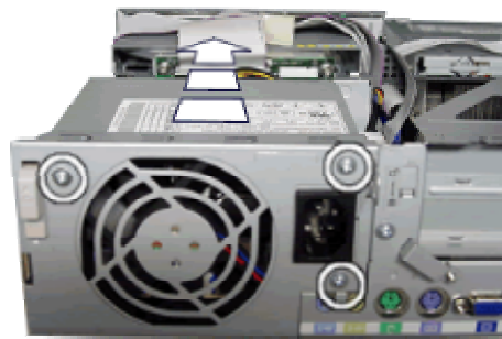
Fig. 16: Removing the screws of the power supply unit
